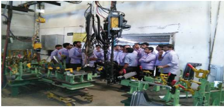
Photo 2: Students observing Pneumatic Systems such as pneumatic gun for spot welding
